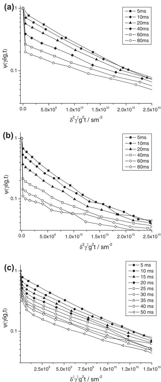
**Fig. 2.** PFG NMR signal attenuation curves with ethane in the purely microporous zeolite (NaCaA-0, (a)) and with ethane (b) and cyclohexane (c) in the mesoporous zeolite (NaCaA-5), recorded at 25 °C.
