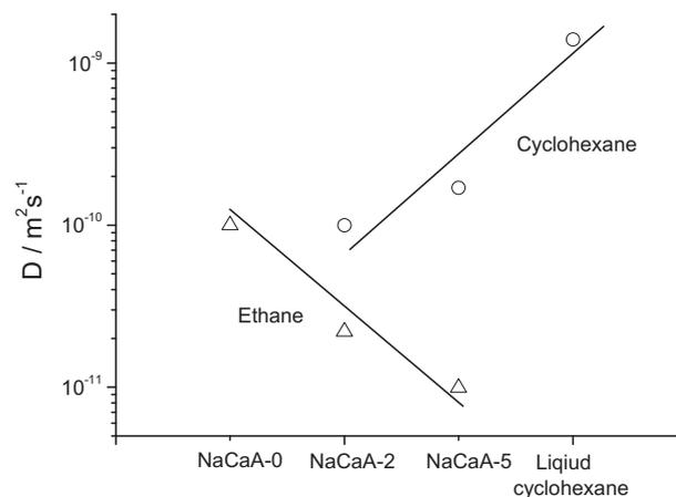
Fig. 4. Comparison of the diffusivity in the space of micropores (probed with ethane; triangles) and mesopores (cyclohexane; circles) of the mesoporous zeolite NaCaA at room temperature. Given, for comparison, are also the diffusivities of ethane in the purely microporous zeolite and of cyclohexane in the neat liquid. The lines are shown to guide the eye.
