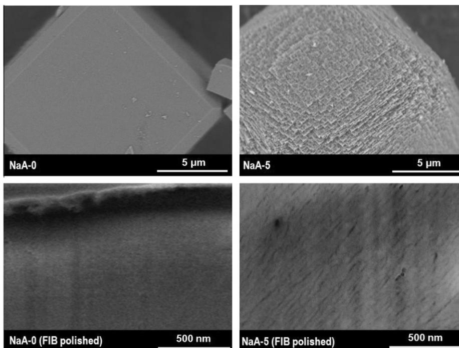
**Fig. 1.** SEM images of the purely microporous (NaA-0, left column) and a mesoporous (NaA-5, right column) LTA zeolite sample: top images were taken from the external surfaces of the calcined samples and the bottom images were taken after cross-sectional polishing by focused gallium ion beam. The dark, slant lines in the lower right image indicate the presence of mesopores in the cross-sectional cut.
