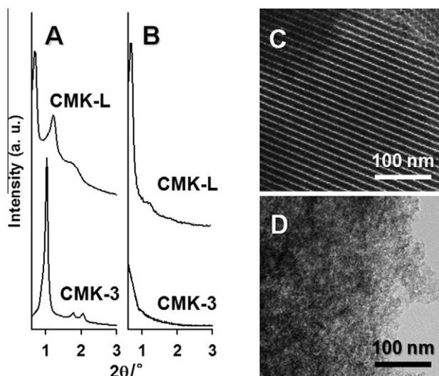
Fig. 6. XRD patterns of (A) carbon templates before zeolite crystallization, (B) after crystallization and TEM micrographs of (C) CMK-L, and (D) CMK-3 after crystallization.
