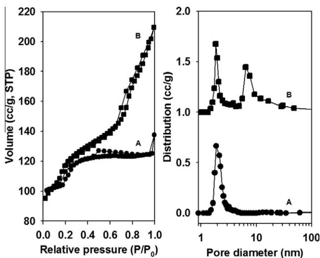
Fig. 3. Nitrogen adsorption isotherms and pore size distributions of (A) Silicalite-1 and (B) SiO<sub>2</sub>/CMK-L at 85% relative humidity. The pore size distribution for SiO<sub>2</sub>/CMK-L at 85% humidity was vertically offset by 1 cm<sup>3</sup>/g.
