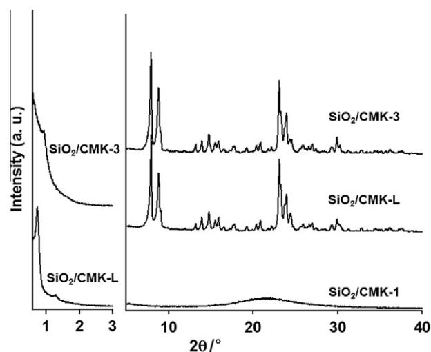
**Fig. 5.** XRD patterns of SiO<sub>2</sub>/CMK-*n* samples using mesoporous carbon templates with various pore structures. The letter after hyphen 'n' denotes the mesoporous carbon template CMK-*n*.
