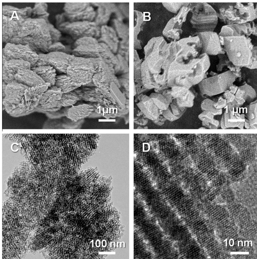
Fig. 2. SEM micrographs of SiO<sub>2</sub>/CMK-L at (A) 85%, (B) 100% relative humidity and TEM images of (C, D) SiO<sub>2</sub>/CMK-L at 85% relative humidity.
