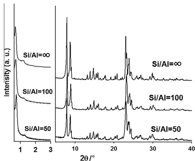
**Fig. 4.** Powder XRD patterns of aluminum containing MFI zeolites synthesized by using CMK-L template (Al<sub>x</sub>Si<sub>1-x</sub>O<sub>2</sub>/CMK-L) with various Si/Al ratios in the range of 50–∞.
