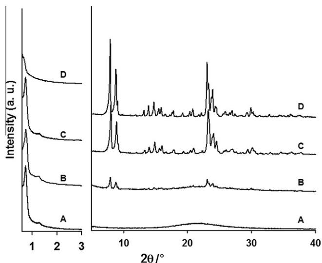
**Fig. 1.** Powder XRD patterns of MFI zeolites ( $SiO_2/CMK-L$ ), synthesized by following dry-gel conversion method at (A) 30%, (B) 50%, (C) 85%, and (D) 100% relative humidity.
