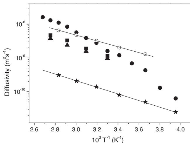
Fig. 4. Arrhenius plot of diffusivities of water in Na-BEA-0 (triangles), Na-BEA-2 (squares) and Na-BEA-5 (filled circles). For comparison, diffusivities of bulk water (open circles, line shows fit of the Arrhenius equation to the data with  $E_A = 16.5 \text{ kJ mol}^{-1}$ ) and water in NaX zeolite (stars, line shows fit of the Arrhenius equation to the data with  $E_A = 18.7 \text{ kJ mol}^{-1}$ ).
