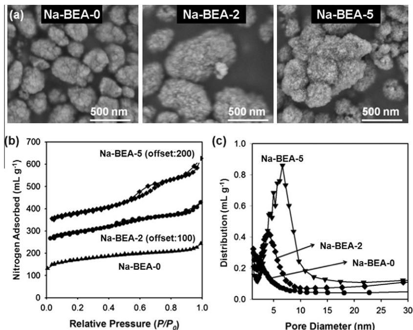
**Fig. 1.** (a) SEM images of Na-BEA zeolite samples with different mesoporosity, (b)  $N_2$  adsorption isotherms of Na-BEA zeolite samples at 77 K and (c) corresponding BJH mesopore size distributions.
