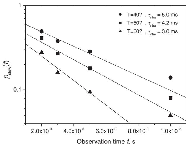
**Fig. 6.** Water diffusion in Na-LTA-2: The relative fraction  $p(t)$  of the slowly decaying component of the PFG NMR spin-echo attenuation (see Fig. 5 for the representation at 50 °C) as a function of observation time  $t$  obtained at different temperatures 40 (circles), 50 (squares) and 60 °C (triangles). The lines show fits of the exponential function to the data at short times  $t$  with the time constants  $\tau_{\text{intra}}$  indicated in the inset.
