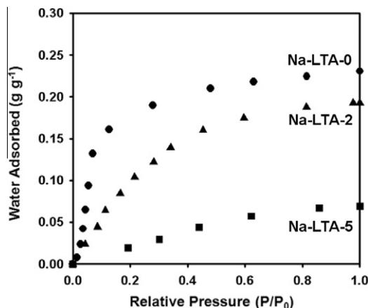
Fig. 3. Water adsorption isotherms of Na-LTA zeolite samples at 300 K which were measured by using gravimetric analysis system.
