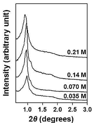
**Fig. 5** Powder XRD patterns for phenylene-bridged PMO materials obtained using 0.034 P123/ $x$  HCl/0.5 BTEB/2.72 BuOH/400 H<sub>2</sub>O. The molar ratio of HCl ( $x$ ) was varied at  $x = 0.25, 0.50, 1.0,$  and  $1.5$ , giving [HCl] = 0.035, 0.070, 0.14, and 0.21 M, respectively.
