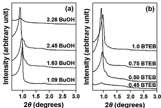
**Fig. 6** (a) Powder XRD patterns for phenylene-bridged PMO materials obtained using 0.034 P123/1.0 HCl/0.5 BTEB/ $z$  BuOH/400 H<sub>2</sub>O, with various molar ratios of BuOH ( $z$ ). (b) Powder XRD patterns for phenylene-bridged PMO materials obtained using 0.034 P123/1.0 HCl/ $y$  BTEB/2.72 BuOH/400 H<sub>2</sub>O, with various molar ratios of BTEB ( $y$ ).
