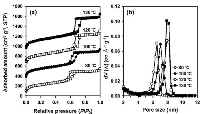
**Fig. 8** (a) Nitrogen adsorption-desorption isotherms for surfactant-extracted PMO-KIT-6-*x* samples. The isotherms for PMO-KIT-6-100, PMO-KIT-6-120 and PMO-KIT-6-130 are offset by 300, 600 and 900 cm<sup>3</sup> g<sup>-1</sup>, respectively, for clarity. (b) NLDFT pore size distribution curves calculated from the isotherms shown in (a) (NLDFT equilibrium conditions - desorption branch).
