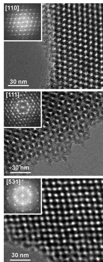
**Fig. 2** TEM images of the cubic  $Ia\bar{3}d$  phenylene-bridged periodic mesoporous organosilica taken with the incident beam parallel to the [110], [111] and [531] directions. The insets are the corresponding Fourier diffractograms.
