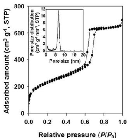
**Fig. 4** Nitrogen adsorption-desorption isotherm measured at  $-196\text{ }^{\circ}\text{C}$  for PMO-KIT-6(1)-100-E. Inset shows the BJH pore size distribution obtained from the adsorption branch of the isotherm.
