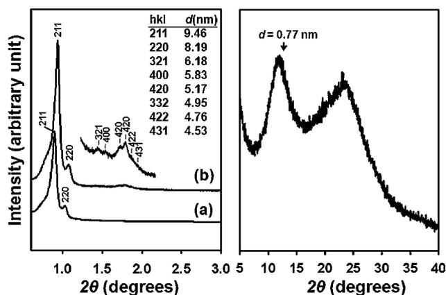
**Fig. 1** (Left) Low angle powder XRD patterns for (a) as-synthesized and (b) surfactant-extracted cubic  $Ia\bar{3}d$  phenylene-bridged PMO material by ethanol, PMO-KIT-6-(1)-100-E. (Right) Wide-angle powder XRD pattern for PMO-KIT-6-(1)-100-E.
