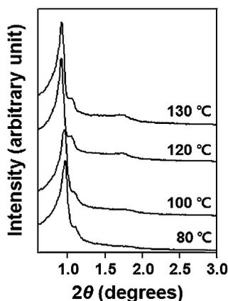
**Fig. 7** Powder XRD patterns for phenylene-bridged PMO materials obtained using 0.034 P123/1.0 HCl/0.5 BTEB/2.59 BuOH/400 H<sub>2</sub>O, at various temperatures of hydrothermal treatment (PMO-KIT-6-*x*, *x* refers to the temperature of hydrothermal treatment).
