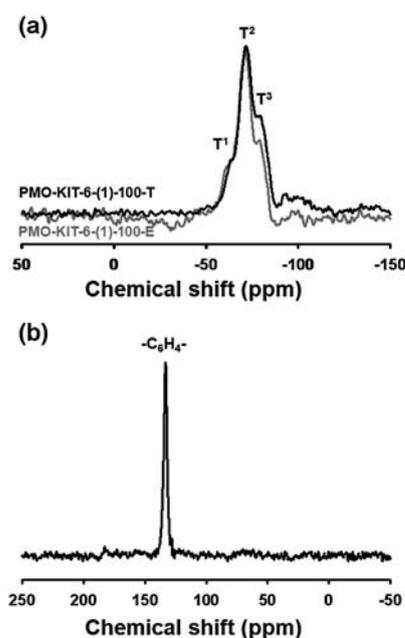
**Fig. 3** (a) Solid state  $^{29}\text{Si}$  MAS NMR spectra for the surfactant-free cubic  $Ia\bar{3}d$  phenylene-bridged PMO materials, ethanol-washed PMO-KIT-6-(1)-100-E (gray) and thermally treated PMO-KIT-6-(1)-100-T (black) and (b)  $^{13}\text{C}$  CP NMR spectrum for PMO-KIT-6-(1)-100-T.
