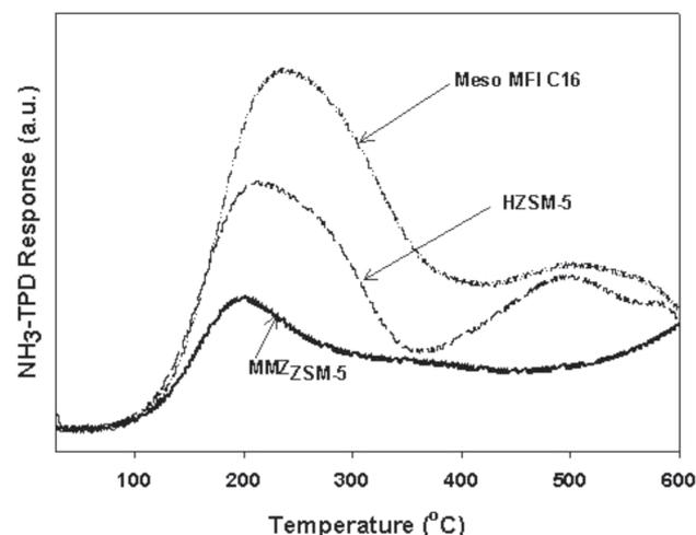
**Fig. 3.** NH<sub>3</sub>-TPD curves of catalysts.**Table II.** Product distribution from catalytic pyrolysis of Japanese larch.
