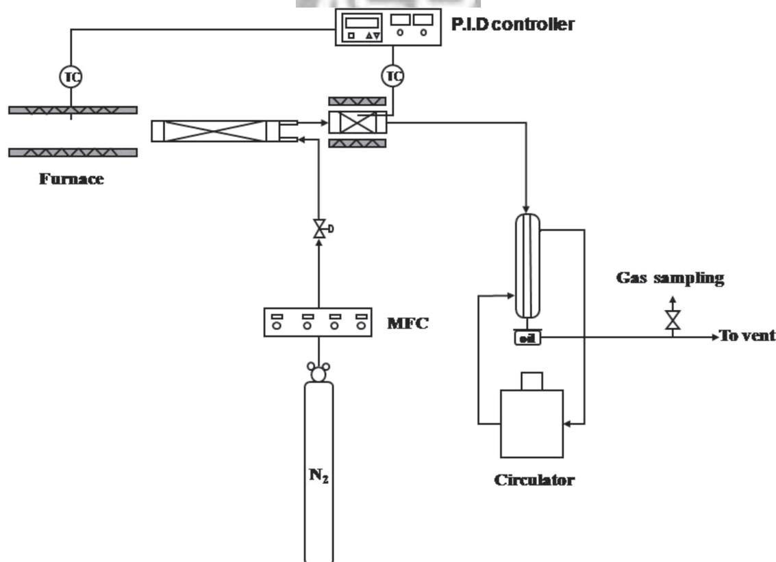
Fig. 1. Schematic diagram of catalytic upgrading apparatus.
