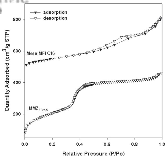
Fig. 2. N<sub>2</sub> adsorption–desorption isotherms of mesoporous catalysts.
