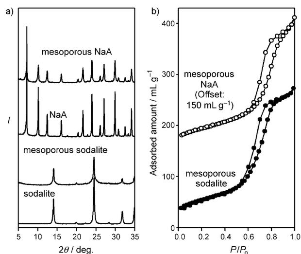
**Figure 1.** a) XRD patterns and b) N<sub>2</sub> adsorption–desorption isotherms of mesoporous sodalite and NaA zeolite.
