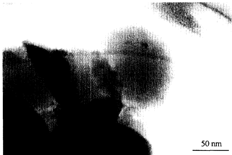
Fig. 2. Transmission electron micrographic image of the hexadecyltrimethylammonium–zirconium oxosulfate mesostructure presented in Fig. 1c.
