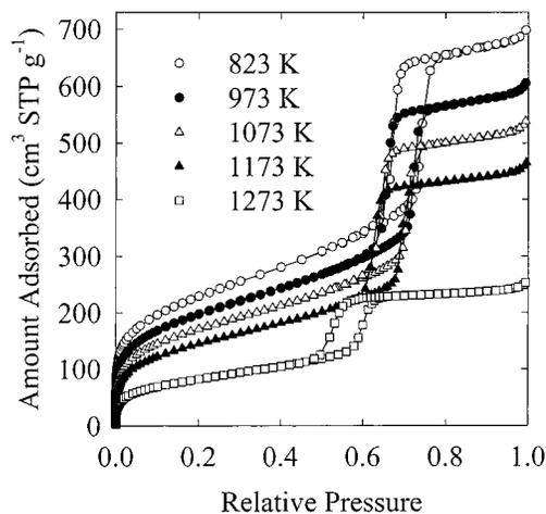
**Figure 7.** Nitrogen adsorption isotherms for the SBA-15 sample B calcined at 823 K and subsequently heated at temperatures up to 1273 K.
