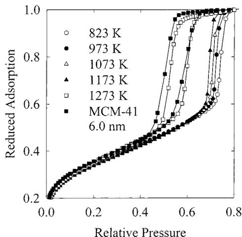
**Figure 9.** Reduced adsorption curves for the SBA-15 sample B calcined at 823 K and subsequently heated at temperatures up to 1273 K. For heat treatments below 1273 K, only adsorption branches of adsorption isotherms are shown. Data for a large-pore MCM-41 are provided for comparison.
