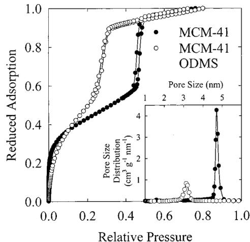
**Figure 5.** Reduced nitrogen adsorption isotherms for the MCM-41 silica, unmodified and chemically modified with ODMS ligands. The inset shows the corresponding pore size distributions.
