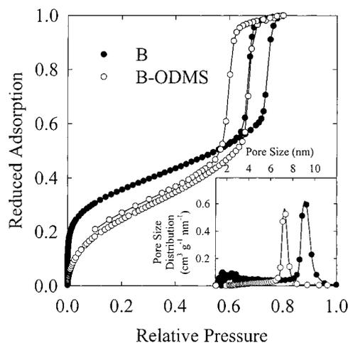
**Figure 3.** Reduced nitrogen adsorption isotherms for the SBA-15 sample B, unmodified and chemically modified with ODMS ligands. The inset shows the corresponding pore size distributions.
