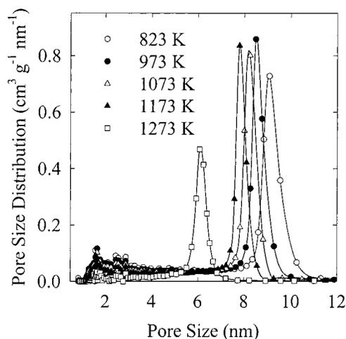
**Figure 8.** Pore size distributions for the SBA-15 sample B calcined at 823 K and subsequently heated at temperatures up to 1273 K.
