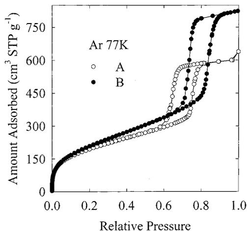
**Figure 4.** Argon adsorption isotherms measured at 77 K for the SBA-15 samples under study.
