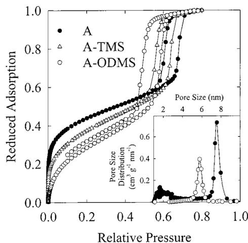
**Figure 2.** Reduced nitrogen adsorption isotherms for the SBA-15 sample A, unmodified and chemically modified with TMS and ODMS ligands. The inset shows the corresponding pore size distributions.
