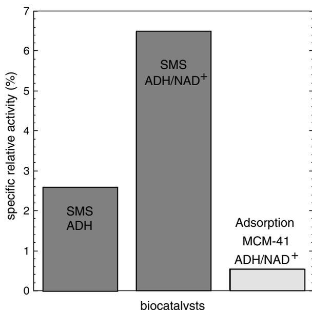
Fig. 11. Relative specific activity of ADH encapsulated in SMS with and without its cofactor NAD<sup>+</sup>. As comparison, relative activity of ADH immobilized with its cofactor NAD<sup>+</sup> by adsorption in a large-pore MCM-41-type.
